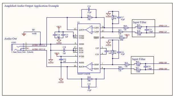
Further noise shaping can be employed by the addition of a DC blocking capacitor between the input filter and the input resistor of the audio amplifier. This forms a high pass filter which has a 3dB cut-off frequency described by the equation below.
