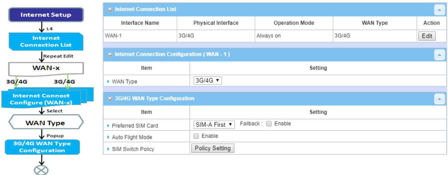
After specifying the physical interface for each WAN connection, administrator must configure their connection profile to meet the dial in process of ISP, so that all client hosts in the Intranet of the gateway can access the Internet.
