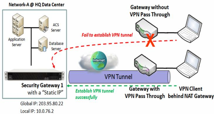
Since VPN traffic is different from that of TCP or UDP connection, it will be blocked by NAT gateway. To support the pass through function for the VPN connections initiating from VPN clients behind NAT gateway, the gateway must implement some kind of VPN pass through function for such application. The gateway support the pass through function for IPSec, PPTP, and L2TP connections, you just have to check the corresponding checkbox to activate it.
