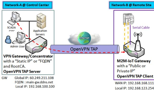
The term "TAP" is referred to bridge mode and operates with layer 2 packets. In bridge mode, the VPN client is given an IP address on the same subnet as the LAN resided under the OpenVPN server. Under such configuration, the OpenVPN client can directly access to the resources in LAN. If you want to offer remote access to the entire remote LAN for VPN client(s), you have to setup OpenVPN in "TAP" bridge mode.
