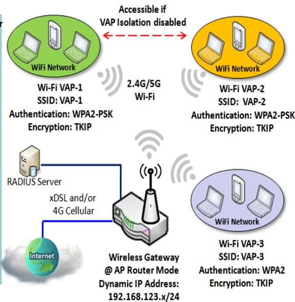
VAP (Virtual Access Point) is function to partition wireless network into multiple broadcast domains. It can simulate multiple APs in one physical AP. This wireless gateway supports up to 8 VAPs. For each VAP, you need to setup SSID, authentication and encryption to control Wi-Fi client access.
