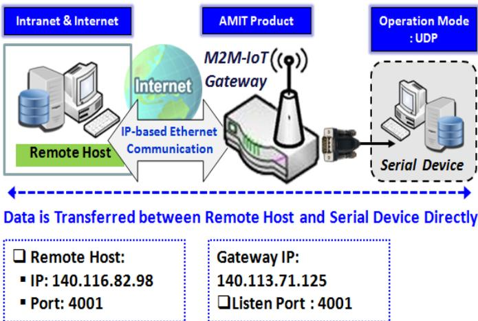
If both the Remote Host Computer and the serial device are expected to initiate a data transfer when it requires doing that, the operation mode for the "Virtual COM" function in the gateway is required to be "UDP". In this mode, the UDP data can be transferred between the gateway and multiple host computers from either peer, making this mode ideal for message display applications.
