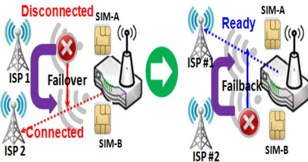
With Failback option enabled, “SIM-A First” scenario is used to connect when the connection is broken, gateway system will switch to use SIM-B. And when SIM-A connection is recovered, it will switch back to use original SIM-A card
