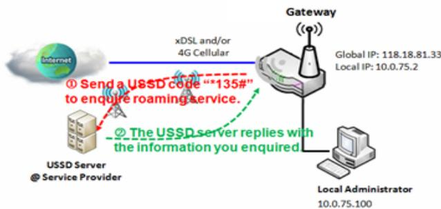
USSD allows you to have an instant bi-directional communication with carrier/ISP. In the diagram, the USSD command **'\*135#'** is referred to data roaming services. After sending that USSD command to carrier, you can get a response at window USSD Response. Please note the USSD command varies for different carriers/ISP.
