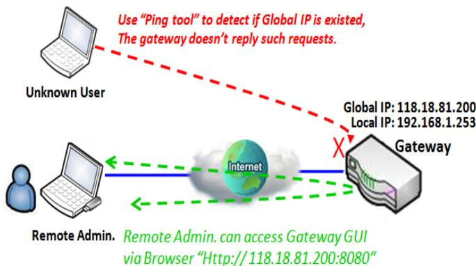
“Discard Ping from WAN” makes any host on the WAN side can't ping this gateway reply any ICMP packets. Enable the Discard Ping from WAN function to prevent security leak when local users surf the internet.
