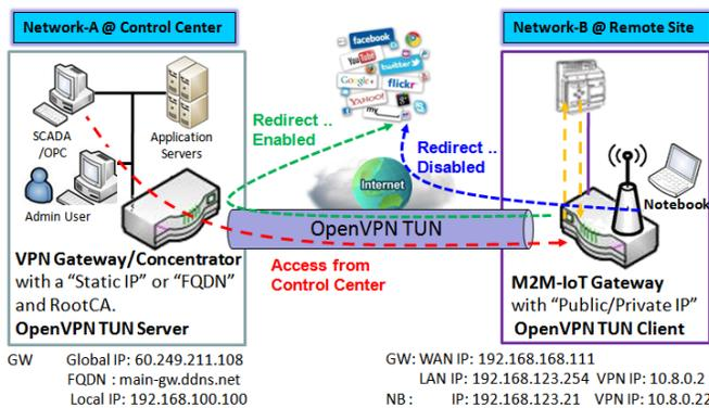
1. M2M-IoT Gateway (as OpenVPN TUN Client) connects to peer VPN Gateway/Concentrator (as OpenVPN TUN Server).
