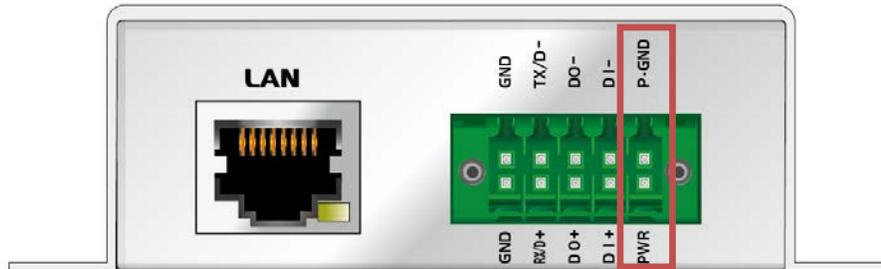
Please connect carefully your power source. Make sure the electrodes have been plugged into the right pins according to their assignments.
