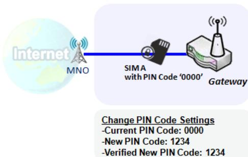
This gateway device allows you to change PIN code on SIM card. Following the example above, you need to type original PIN code “0000”, and then type new PIN code with ‘1234’ if you like to set new PIN code as ‘1234’. To confirm the new PIN code you type is what you want, you need to type new PIN code ‘1234’ in Verified New PIN Code again.
