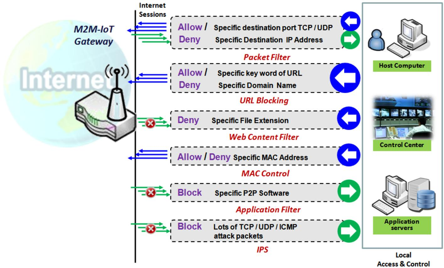
The firewall functions include Packet Filter, URL Blocking, Content Filter, MAC Control, Application Filter, IPS and some firewall options. The supported function can be different for the purchased gateway.
