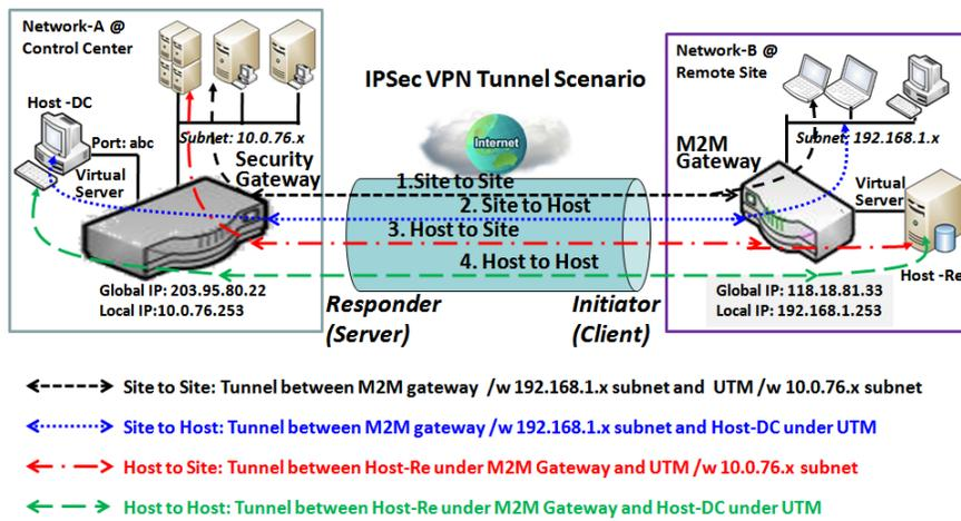
To build IPsec tunnel, you need to fill in remote gateway global IP, and optional subnet if the hosts behind IPsec peer can access to remote site or hosts. Under such configuration, there are four scenarios:
