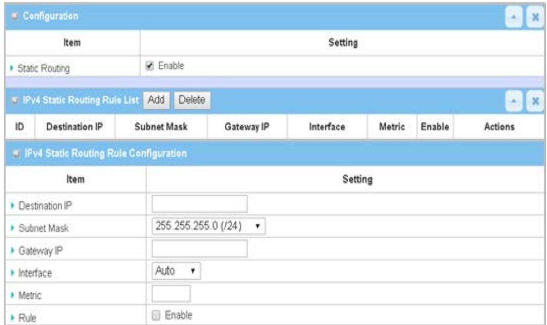
"Static Routing" function lets you define the routing paths for some dedicated hosts/servers or subnets to store in the routing table of the gateway. The gateway routes incoming packets to different peer gateways based on the routing table. You need to define the static routing information in gateway routing rule list.
