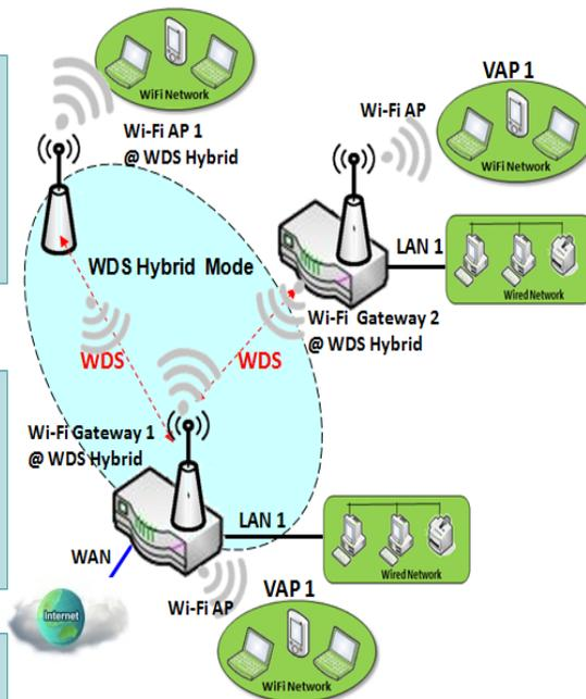
WDS hybrid mode includes both WDS and AP Router mode. WDS Hybrid mode can act as an access point for its WiFi Intranet and a WiFi bridge for its wired and WiFi Intranets at the same time. Users can thus use the features to build up a large wireless network in a large space LAN like airports, hotels or campus.
