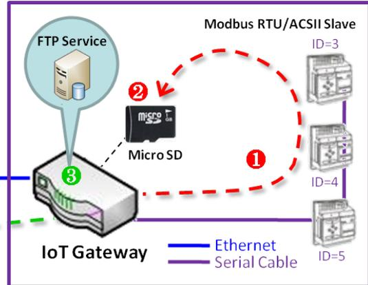
As illustrated, when the connection to a remote Modbus Master broken, the Modbus Gateway will activate the data logging proxy function and execute the pre-defined data acquisition task by itself.
