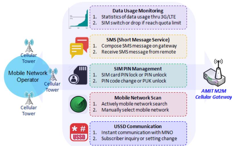
Besides cellular data connection, you may also like to monitor data usage of cellular WAN, sending text message through SMS, changing PIN code of SIM card, communicating with carrier/ISP by USSD command, or doing a cellular network scan for diagnostic purpose.
