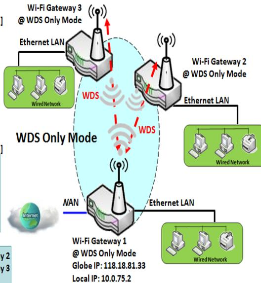
mode. They both use channel 3 to link to local Gateway 1 through WDS. Both gateways connected by WDS need to setup the remote AP MAC for each other. All client hosts under gateway 2, 3 can request IP address from the DHCP server at gateway 1. Besides, wireless Gateway 1 also execute the NAT mechanism for all client hosts Internet accessing.
