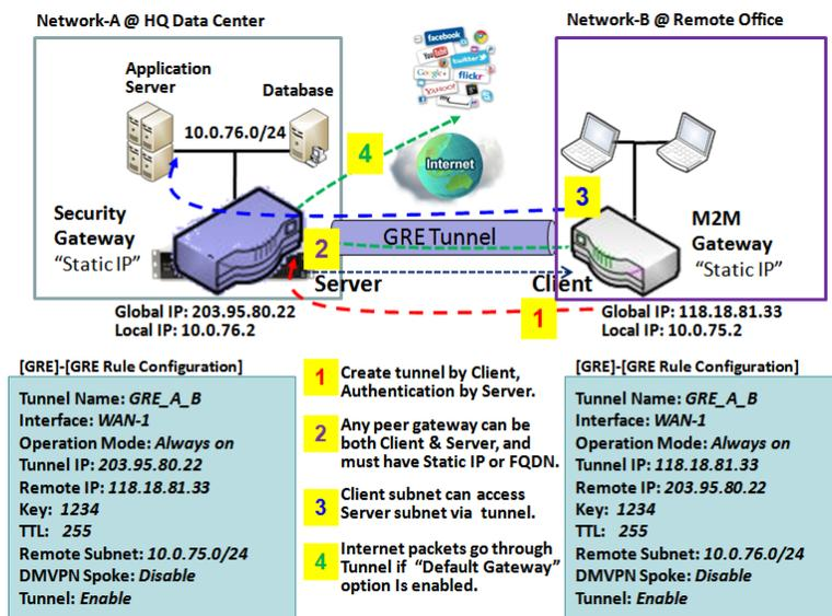
To setup a GRE tunnel, each peer needs to setup its global IP as tunnel IP and fill in the other's global IP as remote IP.
