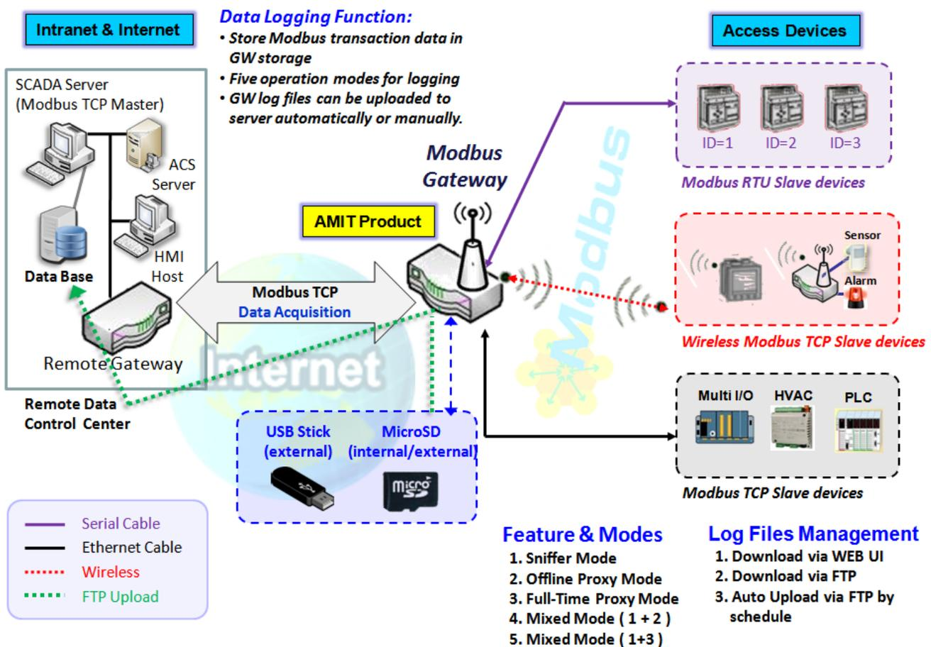
The Modbus Cellular Gateway provides a complete data logging function for collecting the Modbus transaction data for application requirements. There are some data logging schemes to meet different management requirements. They are the Sniffer Mode, Offline Proxy Mode, Full-Time Proxy Mode, and the mixed modes for sniffer and proxy combinations.
