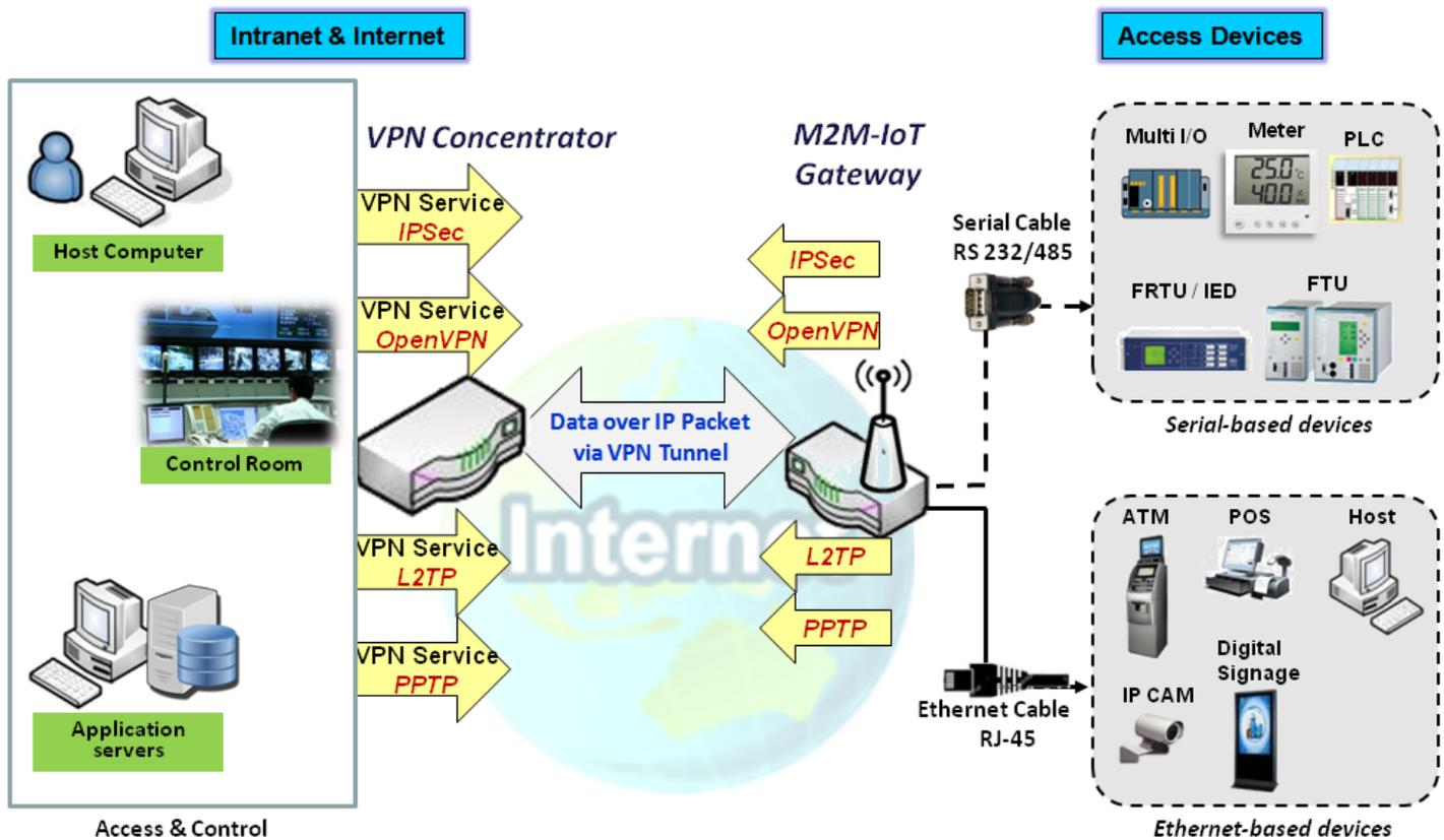
The product series supports different tunneling technologies to establish secure tunnels between multiple sites for data transferring, such as IPsec, OpenVPN, L2TP (over IPsec), PPTP and GRE. Besides, some advanced functions, like Full Tunnel, Tunnel Failover, Tunnel Load Balance, NetBIOS over IPsec, NAT Traversal and Dynamic VPN, are also supported.
