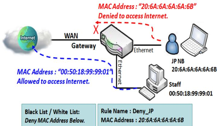
As shown in the diagram, enable the MAC control function and specify the "MAC Control Rule List" is a black list, and configure one MAC control rule for the gateway to deny the connection request from the "JP NB" with its own MAC address 20:6A:6A:6A:6B.
