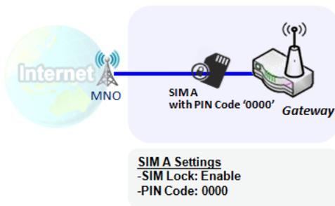
This gateway device allows you to activate PIN code on SIM card. This example shows how to activate PIN code on SIM-A for 3G/4G-1 with default PIN code “0000”.
