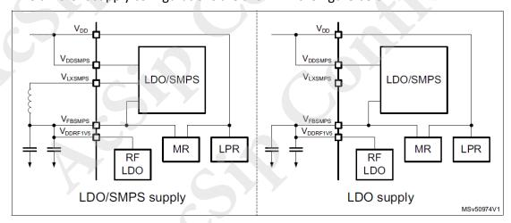
The LDO or SMPS step-down converter operating mode can be configured by one of the following:
