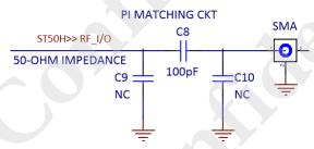
RF SMA CONNECTOR FOR EXTERNAL ANTENNA
