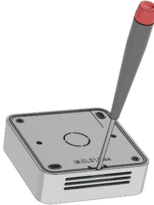
2. Install the batteries. The ERS CO<sub>2</sub> Lite requires one or two AA batteries. The battery type is 3.6V Lithium Battery (ER14505). You can use one battery, but it's recommended that you use two for best performance and battery life. Use battery slot A if only one battery is used.
