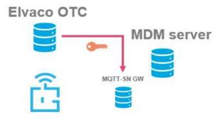
**Step 2:** Device is activated and connects to a bootstrap server (Elvaco's server by default). It receives a pre-shared key for DM-device encryption and IP address to MQTT-SN gateway.
