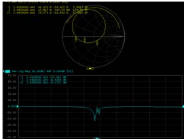
Figure 9: BL652-SA on-board chip antenna performance (Antenna Gain, efficiency and S11 (whilst BL652-SA-xx module on DVK-BL652-xx development board))
