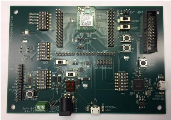
Figure 2: Development board 455-00030 (fitted with 453-00014 EWB module with integrated chip antenna)
