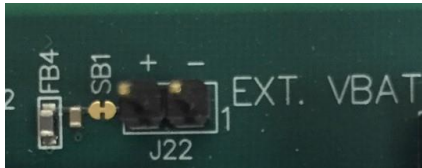
Figure 5: External VBAT power connector
