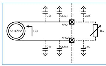
Figure 2: NFC antenna coil tuning capacitors
