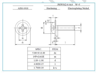
Figure 8: Mounting Screw mechanical drawing
