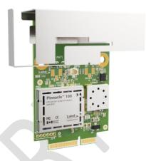
Extremely power conscious, the Pinnacle<sup>™</sup> 100 is ideal for battery-powered devices operating at the edge of your IoT networks, seamlessly bridging the cellular WAN to the BLE network. It's never been easier to bridge wireless Bluetooth 5 sensor data to cloud services like AWS IoT over a low-power LTE connection.
