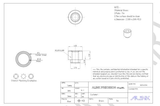
Figure 7: PEM Threaded Standoff mechanical drawings
