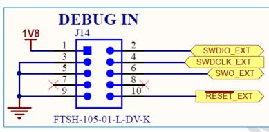
Figure 4: Pinnacle™ 100 development board schematic
