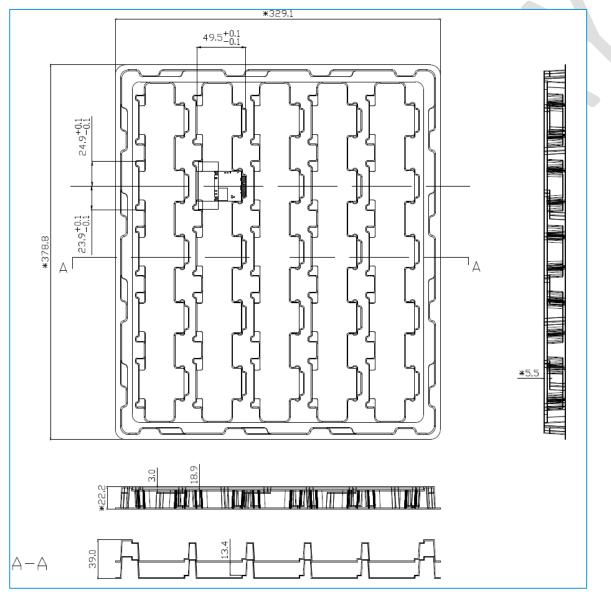
Figure 9: 453-00010 Modem Tray (mm) 25 per Tray
