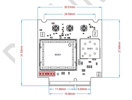
Figure 6: Pinnacle™ 100 453-00011 mechanical drawings
