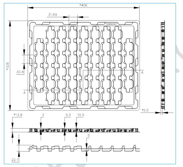
Figure 10: 453-00011 Modem Tray (mm) 50 per Tray
