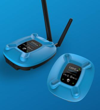
Powered by Laird Connectivity's Pinnacle<sup>™</sup> 100 Modem, the **Sentrius MG100 Gateway** captures data from Bluetooth 5 long range sensors and sends it to the cloud via a global low power cellular (LTE-M / NB-IoT) connection.
