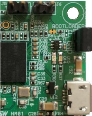
Plug in the micro USB cable. Both the red and green LEDs illuminate at this point to indicate that the unit is in bootloader mode. Remove the jumper from the BOOTLOADER header pin.
