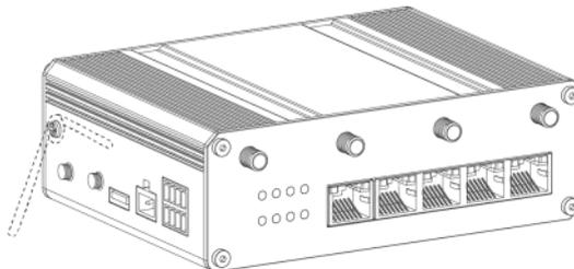
**!** The router must be grounded when deployed. According to operating environment, the ground wire should be connected with grounding stud of router.
