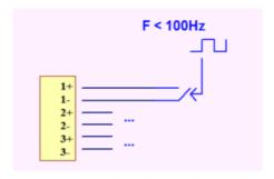
The dry contact must take into account the low polarization current of the input. The use of a silver-or gold-plated contact is recommended to ensure the state is properly detected.
