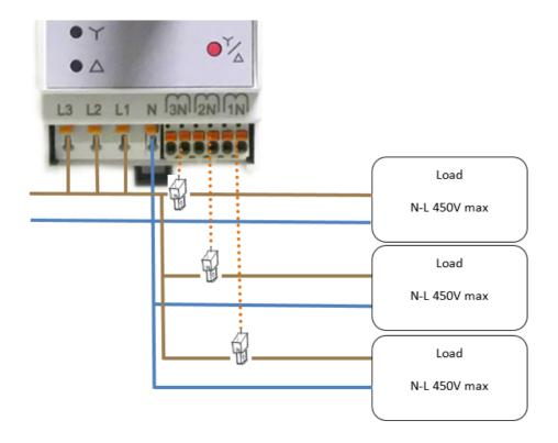
On Mono-phase, it is possible to connect 1 to 3 current transformers on the same phase. If there is more than 1 current transformer then it is necessary to link L1, L2 and L3 to have a measurement of voltage, angle and power of all inputs.
