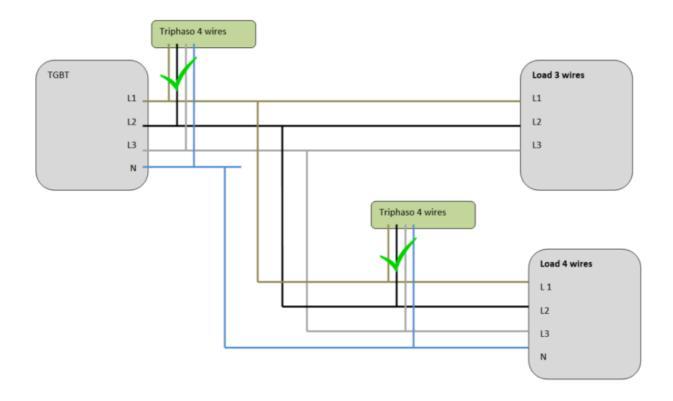
On Three-phase - 4 wires, the Voltage inputs must be connected as following:
