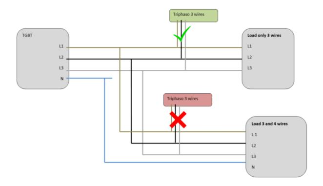
It is not possible to connect Triphaso on 3 wires mode, if there is load behind connected on 3 wires + neutral or on mono-phase. If the Load is not balanced then there is possibility to have current on the neutral which will be not measured by the Triphaso.
