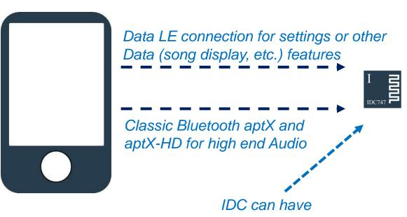
IDC can have simultaneous high end Audio and Data connection with a phone
