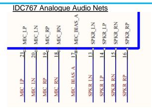
All analogue inputs are DC coupled and must be externally ac coupled for correct operation.
