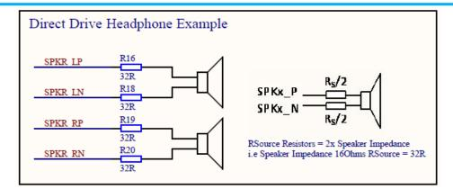
To achieve optimal audio performance in direct drive applications the DACs should operate at close the maximum output voltage of 1Vrms. This can be achieved by adding source resistors between the output terminals and the speaker driver, the value of which are double the rated speaker impedance. i.e., for  $16\Omega$  speakers use  $32\Omega$  resistors, for  $32\Omega$  speakers use  $64\Omega$  resistors.
