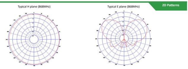
\*Polar Plots measured on a 600x600mm (2'x2') ground plane
