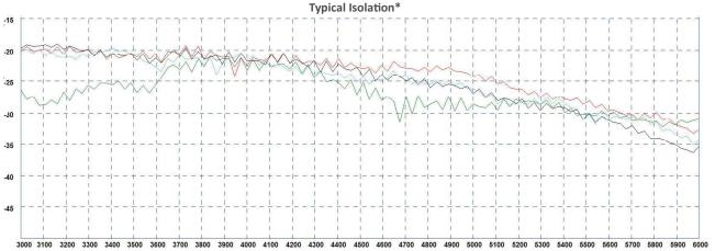
\*Typical Isolation measured with 2m RG174 cable in free space Red Trace = elements 1-2 Green Trace = Elements 1-3 Blue Trace = Elements1-4 Black Trace = Elements 2-3
