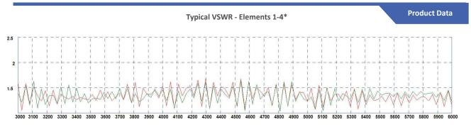
$<sup>^{*}</sup>$  VSWR measured with 2m (6') of RG174 cable in free space - RED TRACE and on a 600x600mm Ground plane - GREEN TRACE
