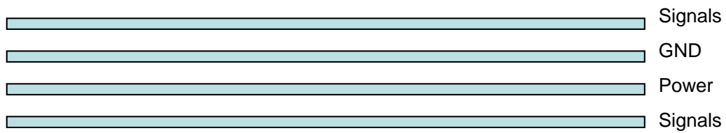
Figure 15: Typical 4-layer PCB construction
