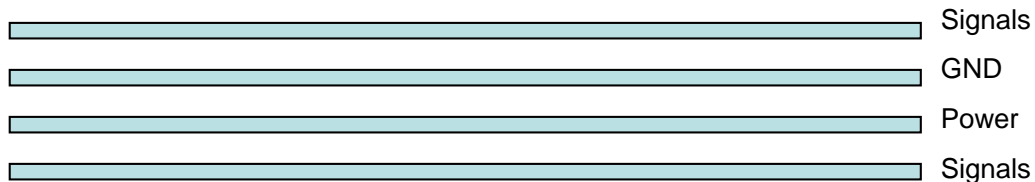
Figure 21: Typical 4-layer PCB construction
