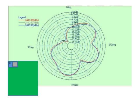
Figure 7: Radiation pattern of BLE113, top view
