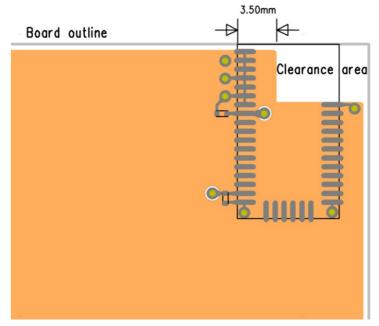
Figure 17: Recommended layout for BLE113-A
