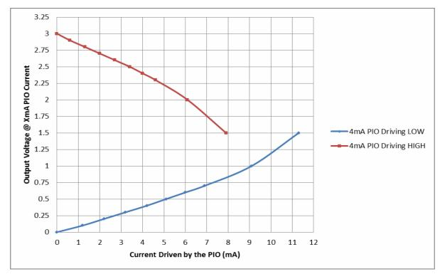
Figure 2: 4mA PIO Current Drive Capability @ VDD=3.0V
