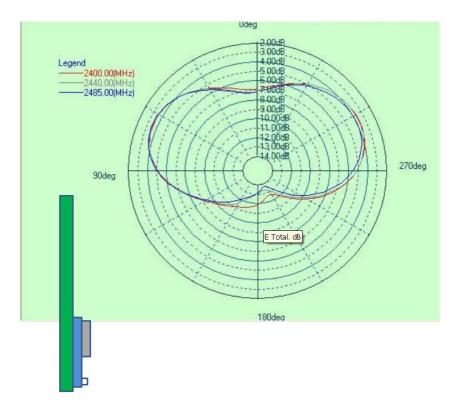
Figure 9: Radiation pattern of BLE113, side view
