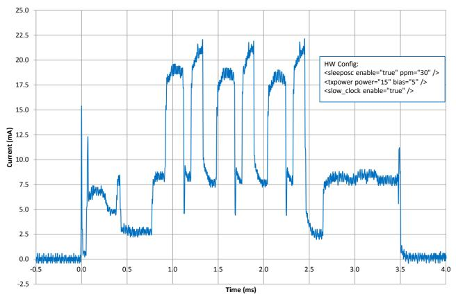
Figure 5: Current consumption profile of BLE113, HR example, advertising
