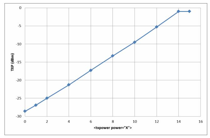
Figure 6: BLE113 TX power as a function of the setting in the HW configuration file
