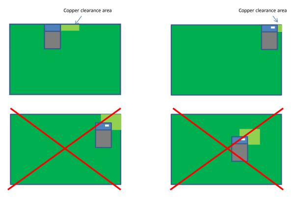
Figure 19: Example layouts for BLE113
