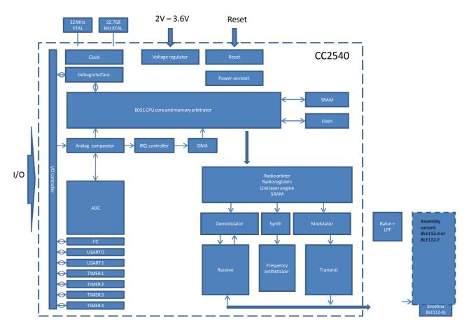
Figure 21: Simplified block diagram of BLE113
