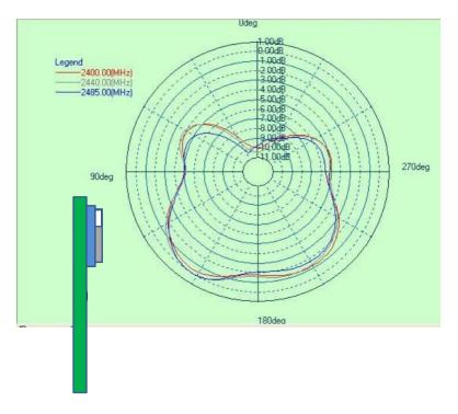
Figure 8: Radiation pattern of BLE113, front view
