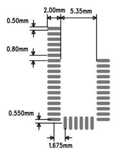
Figure 13: Recommended land pattern for BLE113-A
