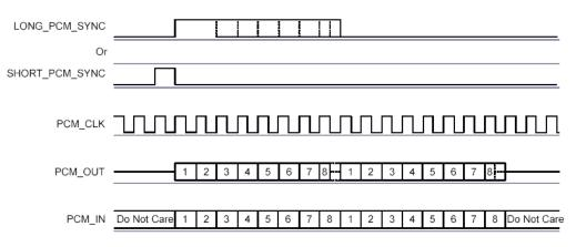
Figure 20: Multi-slot Operation with Two Slots and 8-bit Companded Samples
