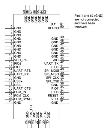
Figure 1: WT41u pin out
