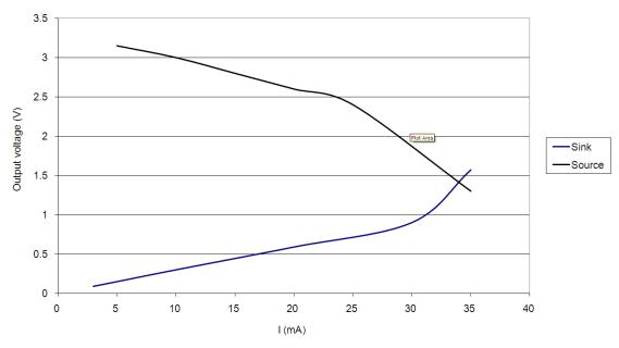
Figure 2: WT41u PIO Current Drive Capability
