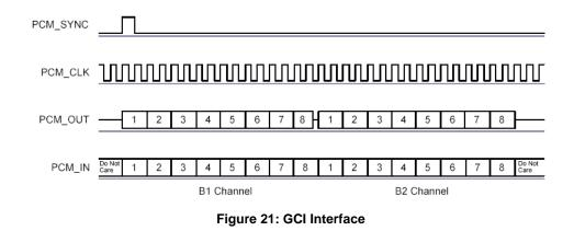
The start of frame is indicated by the rising edge of PCM\_SYNC and runs at 8kHz. With WT41u in Slave mode, the frequency of PCM\_CLK can be up to 4.096MHz.
