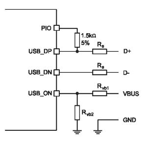
Figure 12: USB Connections for Self-Powered Mode
