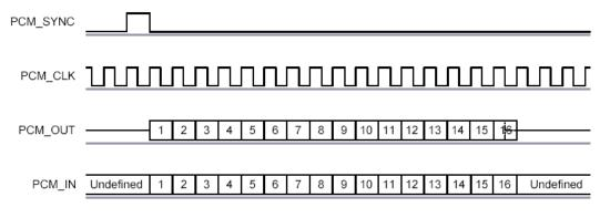
Figure 19: Short Frame Sync (Shown with 16-bit Sample)
