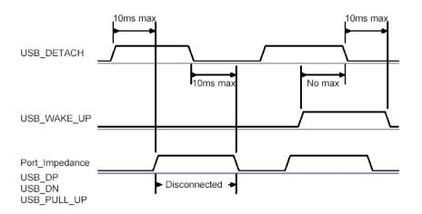
Figure 15: USB\_Detach and USB\_Wake\_Up Signals
