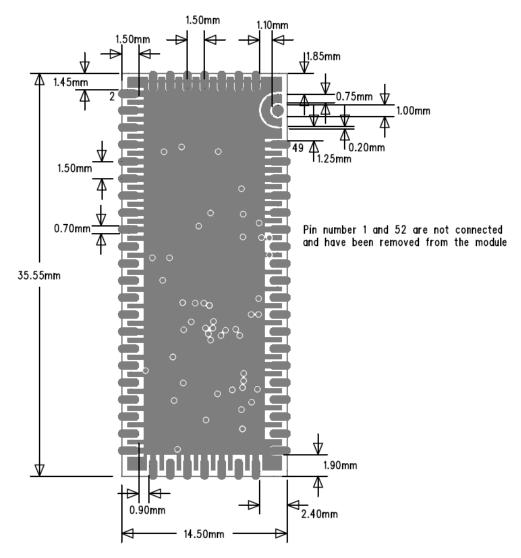
Figure 3: Physical dimensions (top view)
