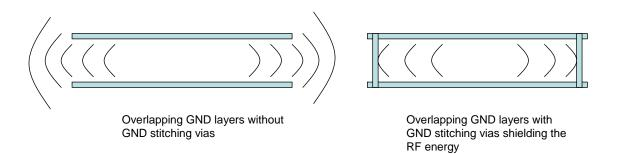
Figure 9: Use of stitching vias to avoid emissions from the edges of the PCB
