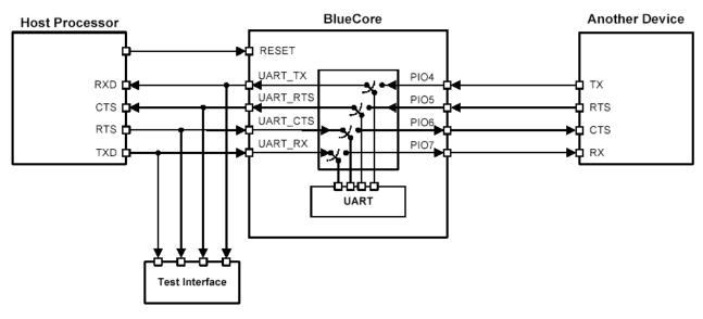
Figure 11: UART Bypass Architecture
