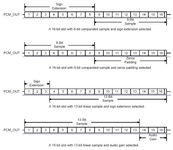
Figure 22: 16-bit Slot Length and Sample Formats
