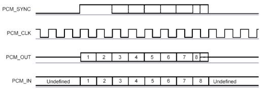
Figure 18: Long Frame Sync (Shown with 8-bit Companded Sample)
