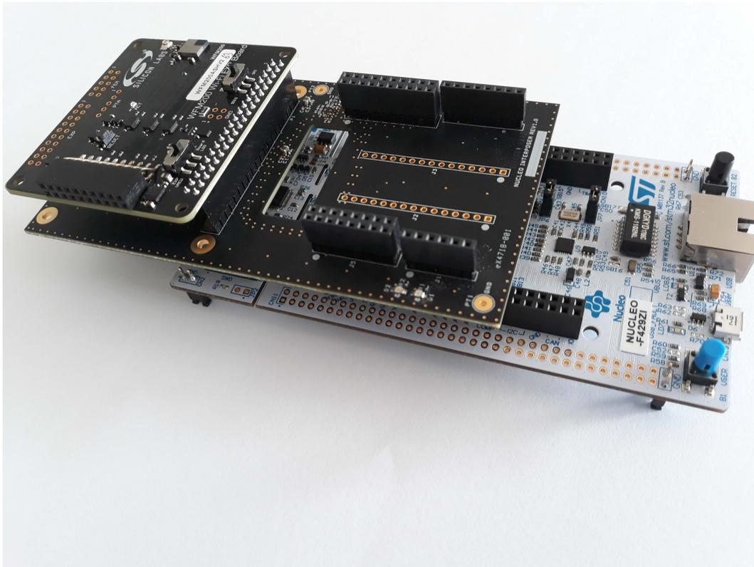
Figure 2.1. WF200 Expansion Board Mounted on a NUCLEO Board
