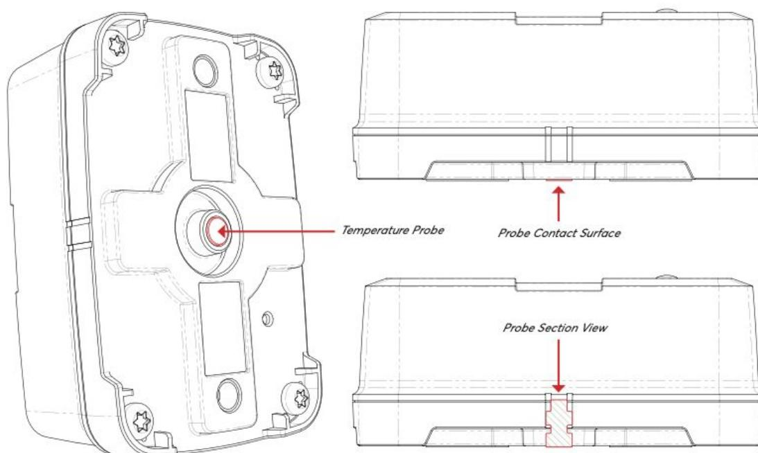
Fig. 12: Temperature Probe
