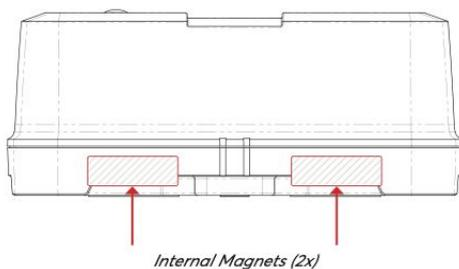
2. For non-magnetic surface peel away the backing of the double sided adhesive and firmly press the sensor onto the surface. Make sure the surface is clean, dust and grease free before mounting.
