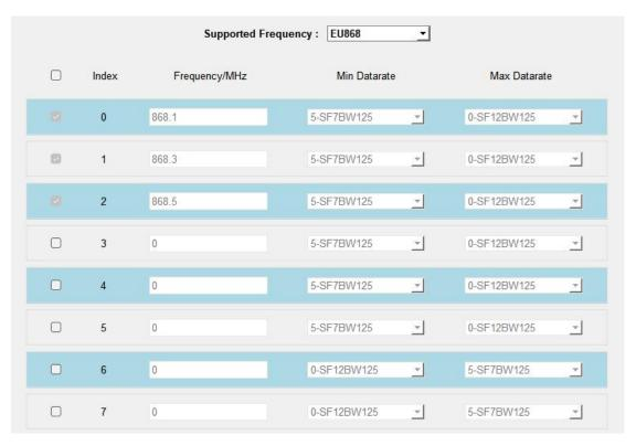
If the frequency is one of CN470/AU915/US915, enter the index of the channel that you want to enable in the input box, making them separated by commas.
