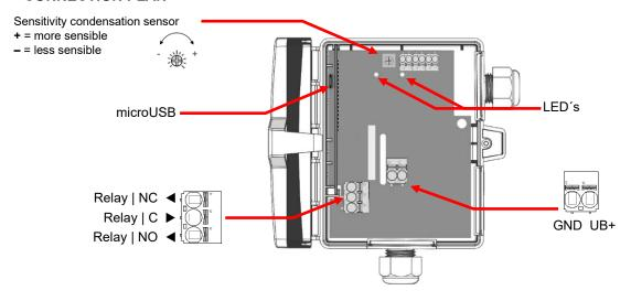
The relay is energized in the operating state (relays NO and C connected). Upon dew permeation or when the operating voltage is switched-off, the relay falls off.
